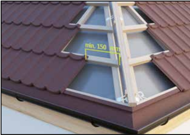
Figure 13. Remember to keep the tile laps staggered. The figures quoted above are given as examples.
