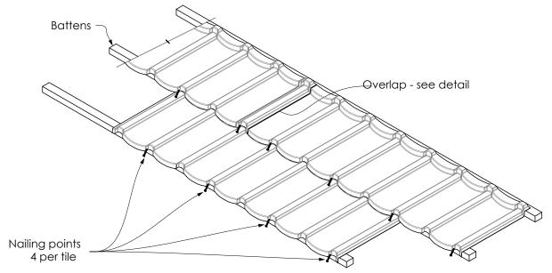
Figure 6.2 Nailing Detail
