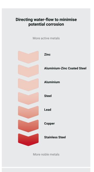
This chart lists commonly used metals in a 'Galvanic Series'. If any two of these metals are in damp contact or a run-off situation, the metal further to the left will sacrifice itself to protect the metal further to the right. Therefore the simple ruleto remember is that Water can flow from top to down.
